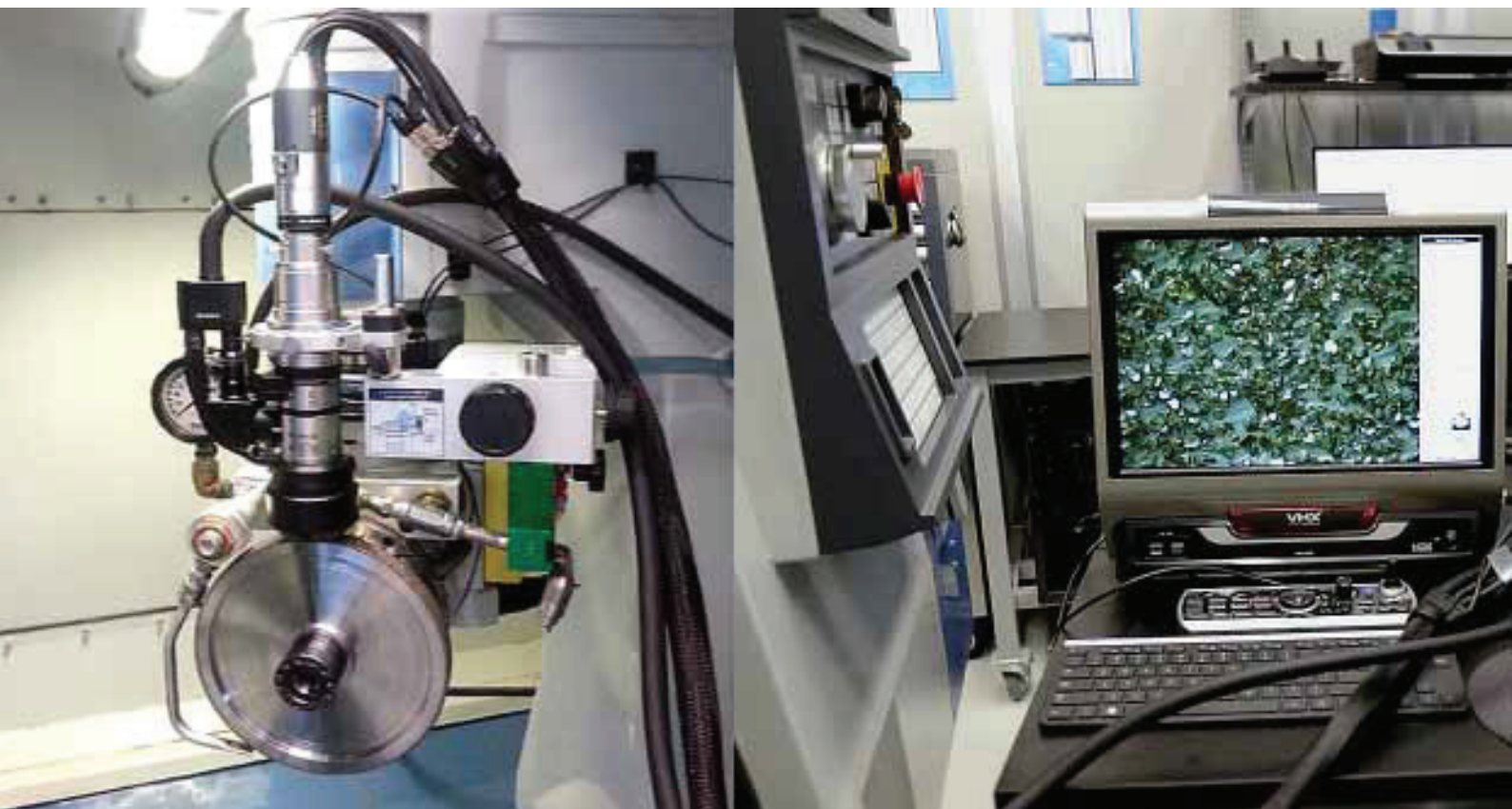
The Keyence VHX 2000 Digital 3D microscope's customized mounting system allows us to take images of the wheel on the spindle.
