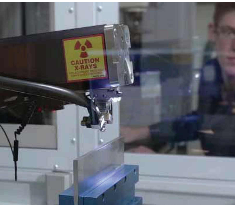
The Proto LXR carefully measures the levels of material stress after grind to provide a closed-loop grinding evaluation.
